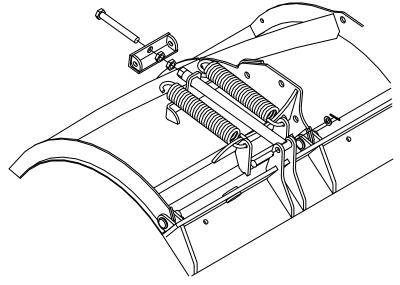
Figure 4. Install Trip Springs
