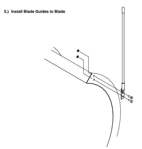
Figure 7. Install Blade Guides
