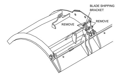
Figure 3. Remove Blade Shipping Brackets
