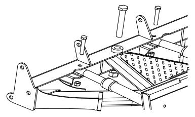
Figure 2. Assemble Pushframe Attachment Bar
