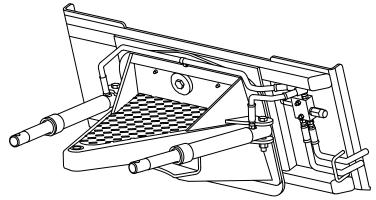
Figure 1. Plow Box Assembly
