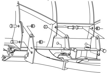
Figure 6. Install Quad assembly to Blade Assembly
